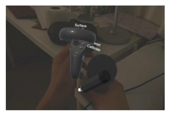
3. **Set Second Point**: Move the pen to the **bottom-right** corner and press the "X / Calibrate" button again.
